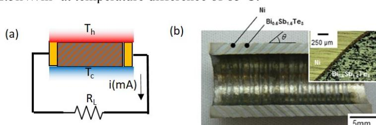
Figure 1(a) Schematic of power generation for transverse thermoelectric material. (b) Prototype device for liquid-liquid heat exchanger from ref 1. Alternating layers of BiSbTe and Nickel.
